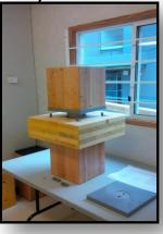
CLT floor slabs with glulam columns and steel connectors
