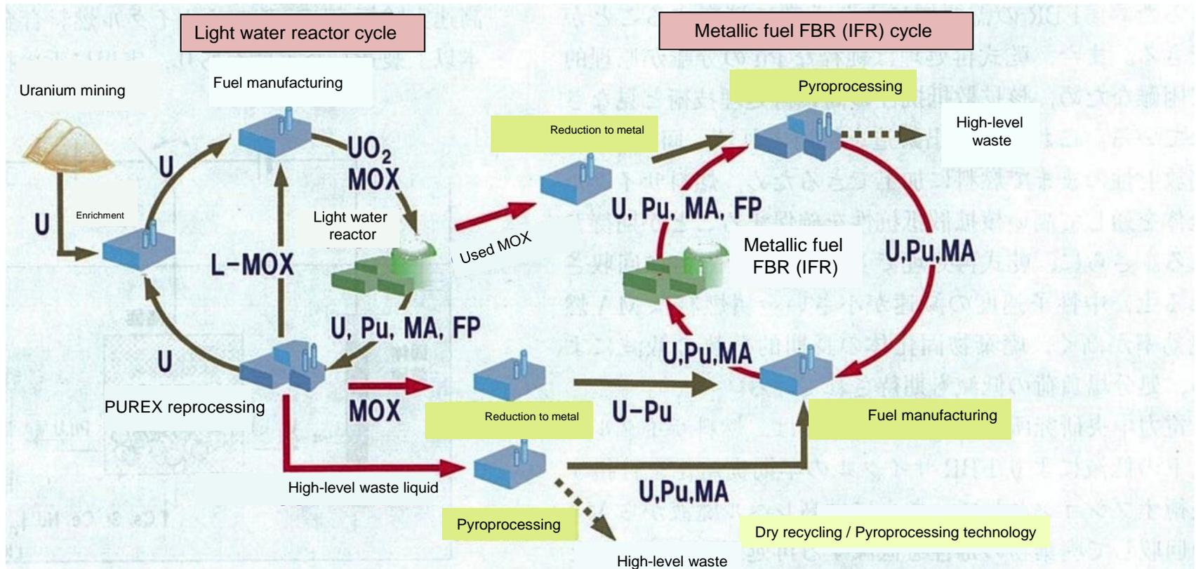
Figure 6: Fuel cycle concept using Pyroprocessing technology
