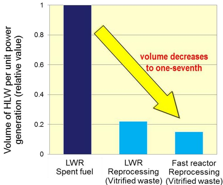
Reduction in the volume of high-level radioactive waste
