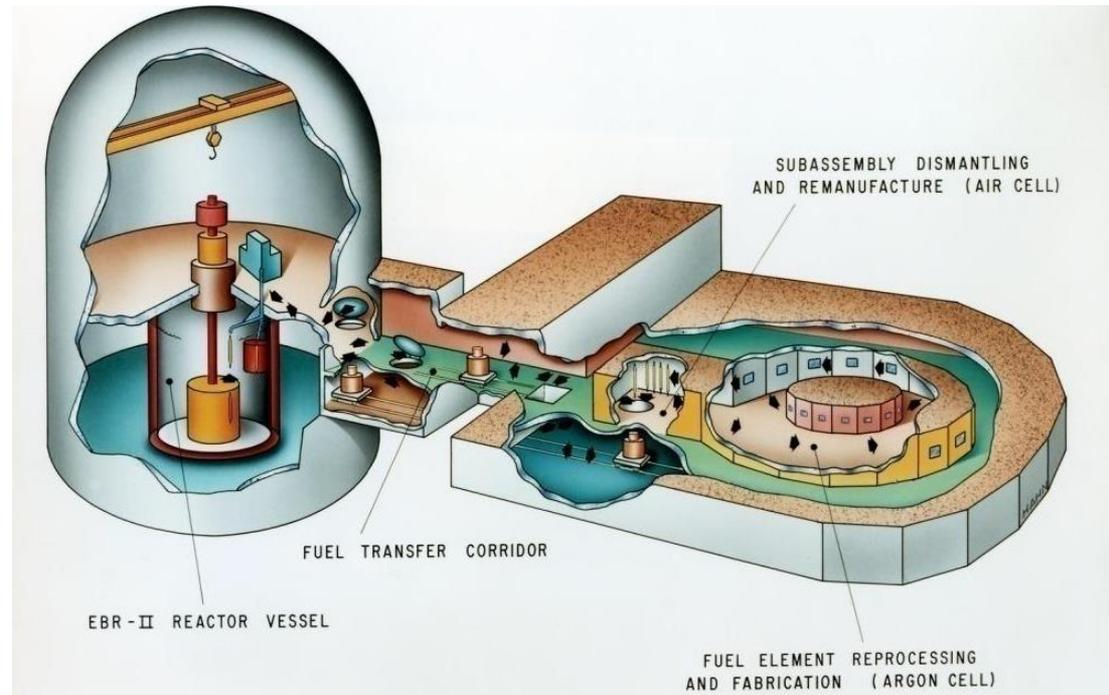
Concept diagram of an IFR that combines a fast reactor with a fuel recycling facility
