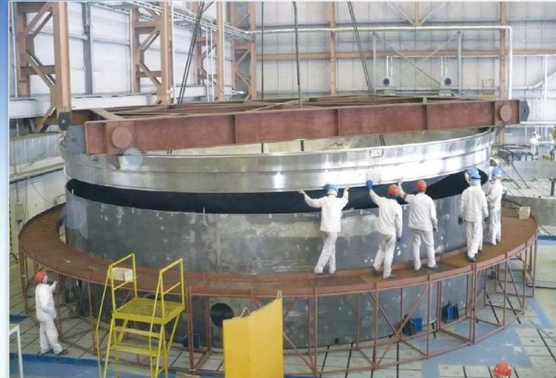
Assembling the reactor vessel's thermal baffles
